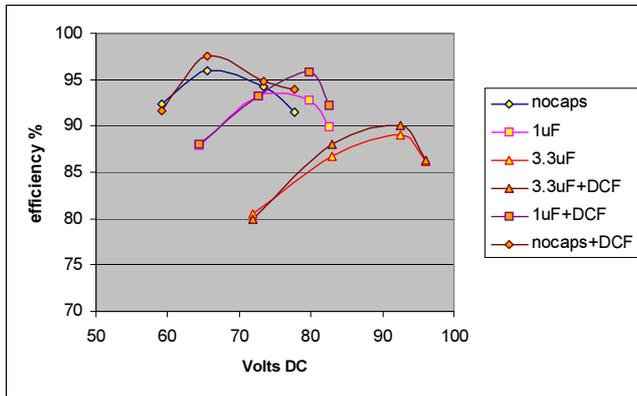
Fig 8. Effect of phase-to-phase capacitance and DC filtering on alternator-rectifier efficiency. DC filtering has a small positive effect on efficiency, but only when alternator operates near the peak efficiency.
