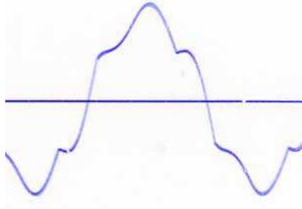
Fig 4. Effect of phase-to-phase capacitors. Voltage spikes are eliminated and both peak and RMS value of the AC phase voltage are increased.
