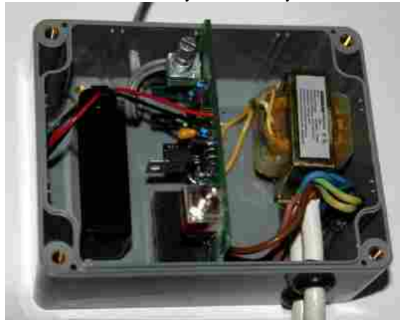
Fig 4. Inside the assembled thermostat. The thermostat enclosure is waterproof. Right: transformer. Left: the 9V NiMh battery.
