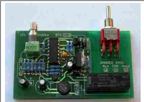
Fig 3. The printed circuit board of the thermostat is double-sided and has insulating solder masks to maximize the circuit safety and reliability.
